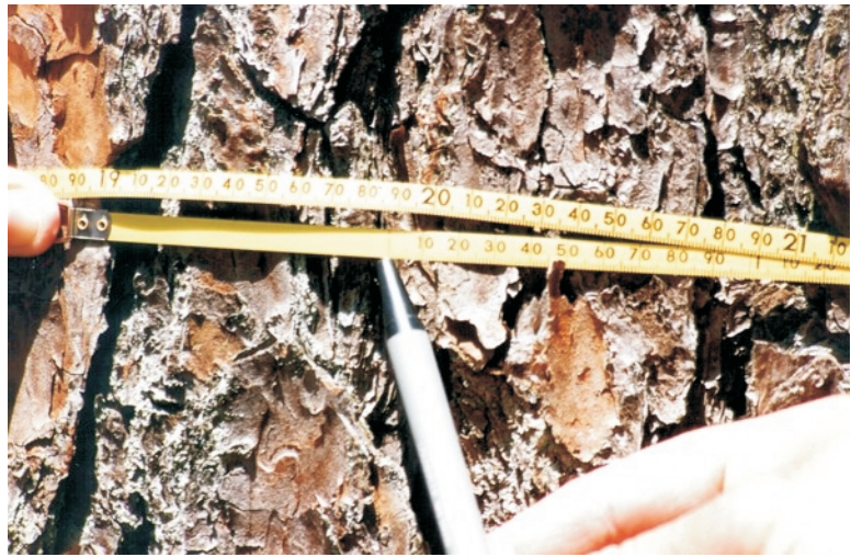
FIGURE 2. The dbh of this tree is being measured with a diameter tape.
